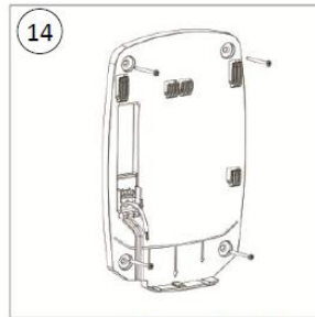
14 Screw the Plug-in base to the wall(x4)
